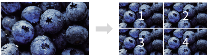
4K 2 Sample Interleave (2SI) : Pixel based segmentation
