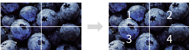
4K Square Division (SQD) : Quadrant based segmentation
