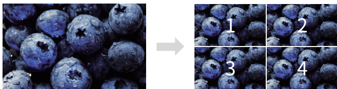
4K 2 Sample Interleave (2SI) : Pixel based segmentation
