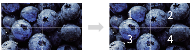
4K Square Division (SQD) : Quadrant based segmentation
