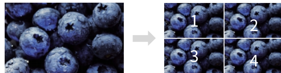
4K 2 Sample Interleave (2SI) : Pixel based segmentation
