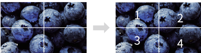
4K Square Division (SQD) : Quadrant based segmentation
