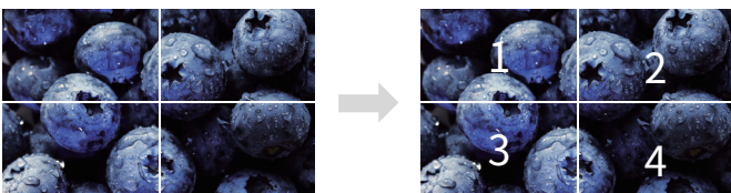
4K Square Division (SQD) : Quadrant based segmentation
