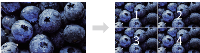
4K 2 Sample Interleave (2SI) : Pixel based segmentation
