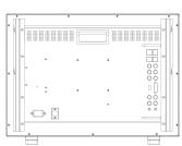
Main Body:570×404.1×111.6(mm) Main Body:570x429.1x149.6(mm)(with rack) Weight:8.40KG
