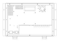
Main Body:433.7×295×122.3(mm) Main Body:465x295x122.3(mm)(with rack) Weight: 5.15KG
